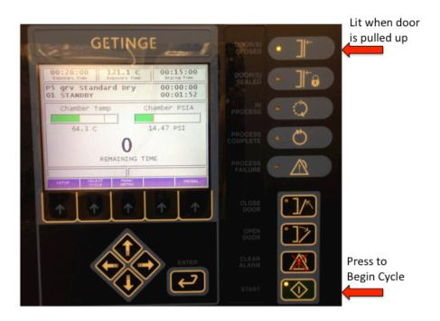
2. **Start** button should be blinking, and **Door Closed** indicator lit. <u>Push **Start** Button.</u>
