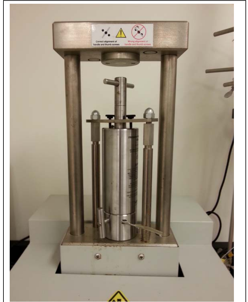
Figure 2: Proper set-up of the cell in the press. Note how the handle is perpendicular to the thumb screws on the cell clamp.
