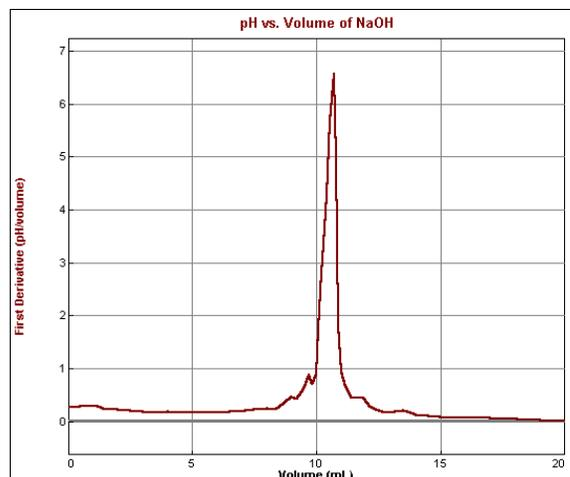
**Figure 2.** First derivative vs. volume for the titration curve shown in Figure 1 (this graph is mistitled). The largest value of the first derivative is at the volume corresponding to the equivalence point (10.7 mL).
