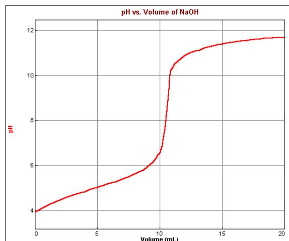
**Figure 1.** A typical titration curve for a weak acid titrated by a strong base (NaOH).
