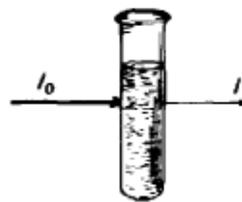
Figure 1. The reduction in light intensity due to absorption by a solution.
