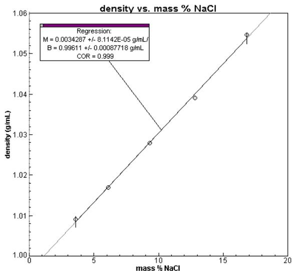
Figure 1. Density vs. mass % NaCl. The best-fit line was added using linear regression.
