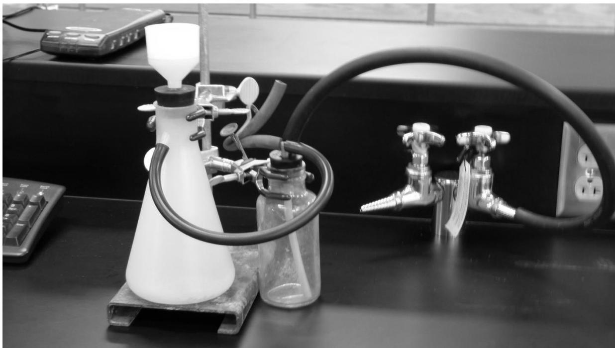
Figure 1. A suction filtration apparatus.
