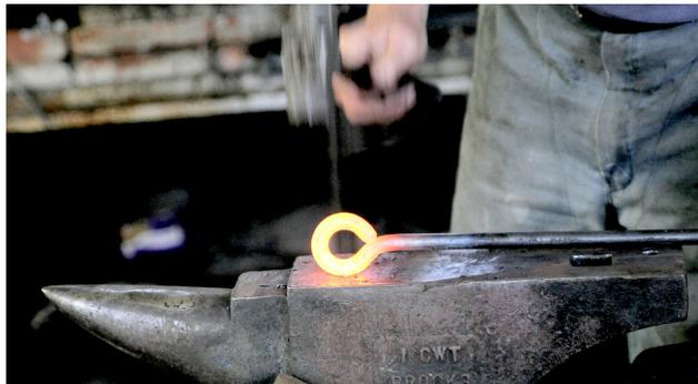
wooden wheels the blacksmith makes an iron hoop whose radius is less than the wheel radius. He heats it enough to mount it around the wheel. When it cools down it grabs the perimeter of the wheel.
